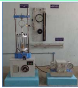
Triaxial Compression Test equipment
